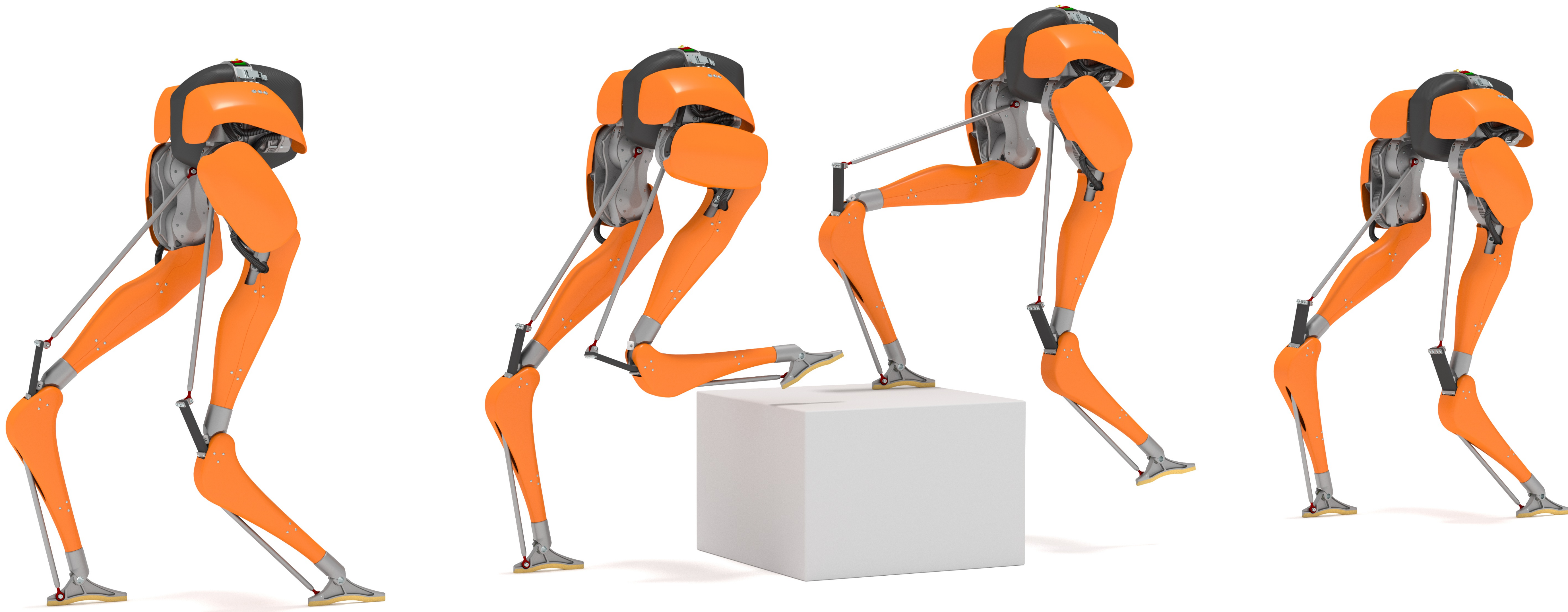
Cassie is an agile bipedal robot built for efficient spring-mass walking and running. Here, Cassie is shown performing a dynamic task that requires planned interaction with the environment. Several logical steps are shown, but what is the action space through which the planner communicates these steps to the controller?
